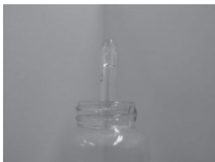
Figure 3. Photograph of the cyclohexane gel of 2 (4.1 wt %) in an NMR tube at 20 °C.
